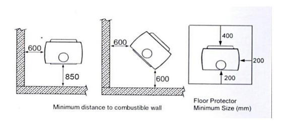
It is recommended that the stove be installed at least 600mm from combustible materials. However, any household furnishings should be at least 1000mm away as they could be adversely affected by heat.
