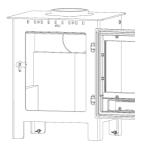
Insert a solid mineral fuel top side brick on the Left hand side of the Stove (Part No: FM5-042).
