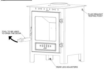
When positioning the stove the two rear legs are fitted with adjustment plates to accommodate for hearth variations.
