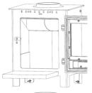
7 Insert the solid mineral fuel burning grate (Part No: FIREM-001).
